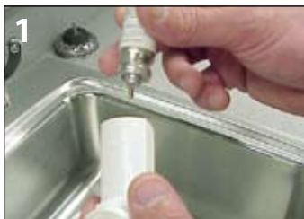
1 Take metal canister out of plastic container.
